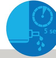
Open the drain valve or tap and allow it to flush briefly (about 5 secs or until hot water is present) before placing the bottle in the water stream. Fill the bottle to the top but try to avoid overflowing.
